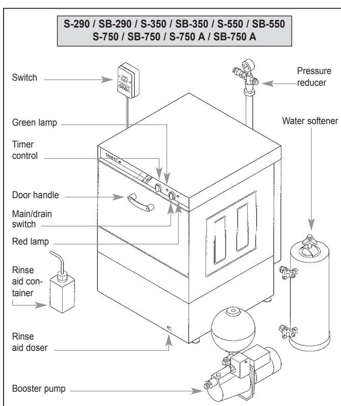
**Important:** Check that the rinsing aid container is filled up. By turning the timer, 7 or 8 impulses, we will see the filling of the rinsing aid tube and its going into the boiler. The doser adjustment is made by means of an adjusting screw.
