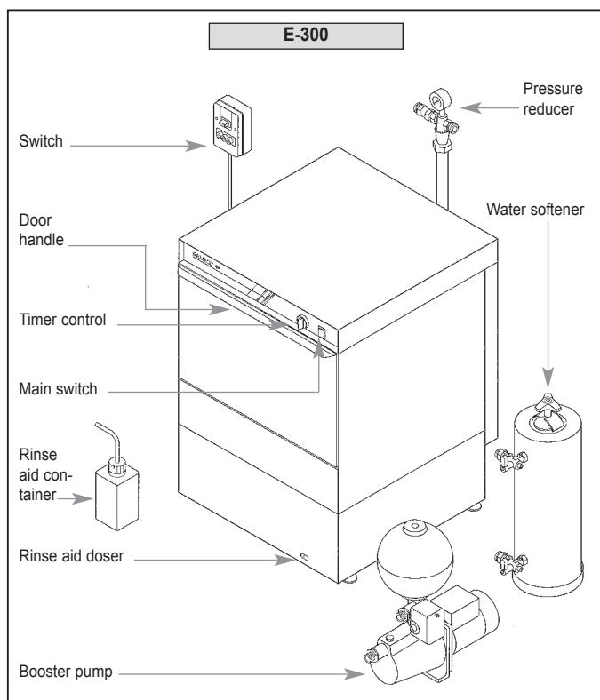
Connect one end of the booster pump to the water cock and the other end to the hose using the thread mouthpiece of the machine.
